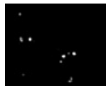
Hydraulic spray on leaf underside. Average count in 54 samples = 6.3 deposits in 1/8 in 2
