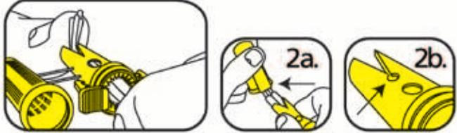
Insert wires through flexible sealing fingers and bend bare wire ends together into one "V-Channel." When connecting heavy solid wires, use bending sleeve / depth gauge on outer sleeve of connector (see illustration 2a). For larger connections (e.g. three #12 wires, or equivalent, or more), bend wires into the V-Channel with round hole at bottom (see illustration 2b); pull folded group of wires downward into this hole at bottom of "V."
