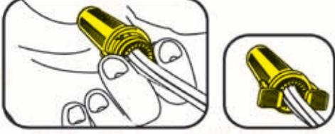
Separate connector, removing plastic "link" or "leg" from inner sleeve. Push inner sleeve into pre-filled outer sleeve until double-locked. Ensure that bending sleeve does not come down over either latch. Pre-filled silicone fully waterproofs the connection. Do not reuse.
